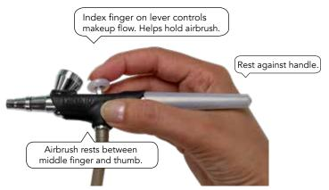
Hold the airbrush as you would hold a pen, with gentle grip and fingers extended. Find a comfortable grip and place your index finger on the lever. Use your index finger to pull back on the lever gently. Never use your thumb to control the lever.
